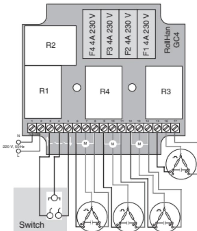
Fig. 2. GC4 group control connection diagram
