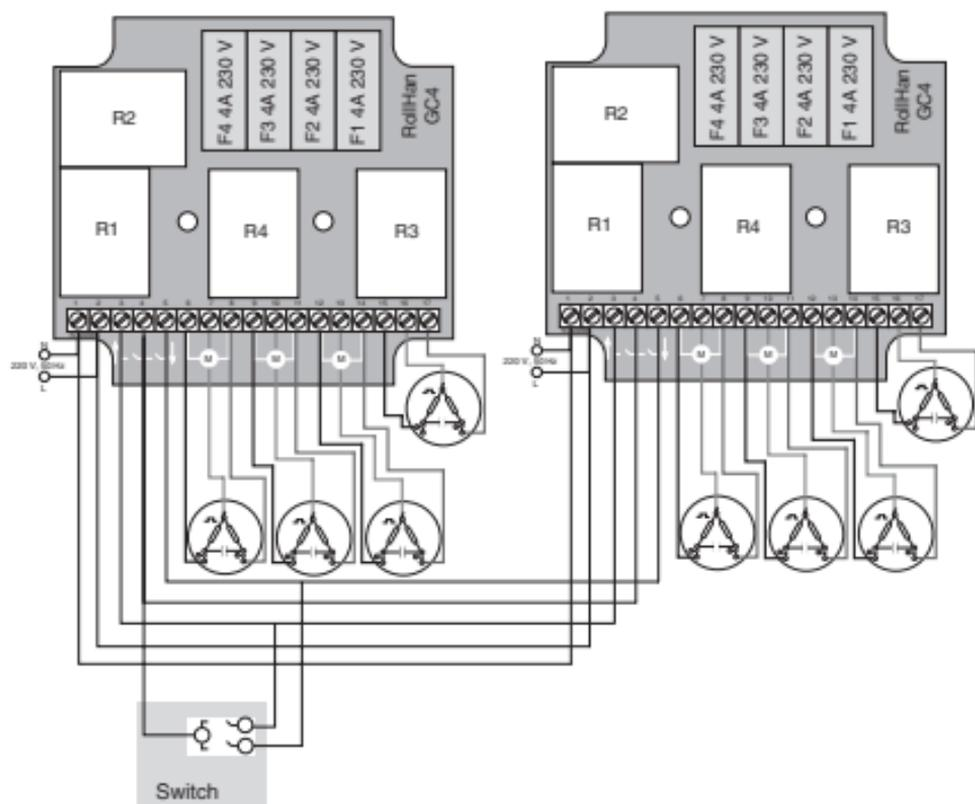
Fig. 3. GC4 block connection diagram
